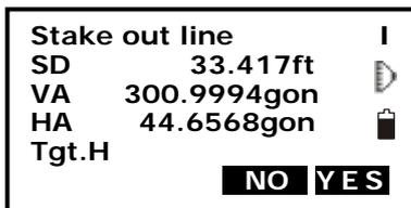
5. Press F3: [NO] to re-measure the target.
