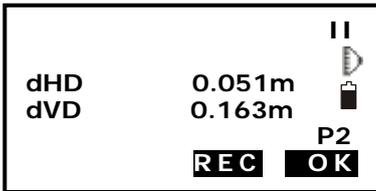
press F3: [REC] to record and set the station, then back to the previous mode. You could also press F4: [OK] to set the station, but the data will not be recorded.
