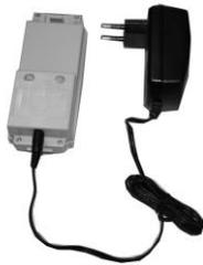
As above figures show, connect the charger and the battery, then plug the charger into the outlet of 100V-240V AC power supply, recharging will begin.
