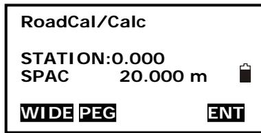
1. Input the interval of staking points on the road.
