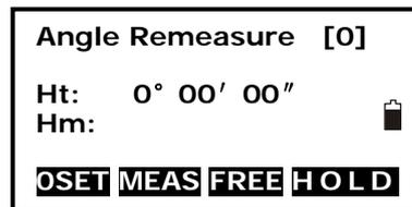
4. Collimate the target A and press the F1[OSET] key.
