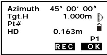
backsight checking, HD between station and backsight, dHD and dVD between calculated backsight and measured backsight will be display.
