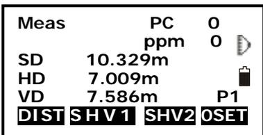
4. Press F3: [SHV2], SD/HD/VD and SD/VA/HA are displayed alternatively.
