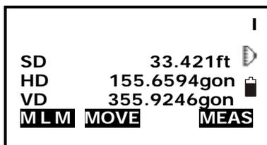
2. Aim at the start point P1, then press F4: [MEAS] and the measured data will display.
