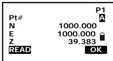
3. Input the data in corresponding items. You could press F1: [READ] to read the existed coordinate data for start point. Press F4: [OK] to enter.
