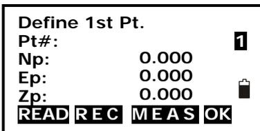
5. Input the first point data, or press F1: [READ] to use existed coordinates data, or press F3:[MEAS] to measure the point.
