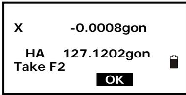
5. Rotate the instrument 180°/200gon. Loosen the horizontal clamp and turn the instrument 180°/200gon while referring to the displayed horizontal angle, then re-tighten the clamp. Wait a few seconds for the display to stabilize, then read the automatically compensated angles X2 and Y2.
