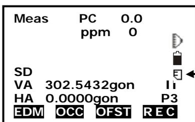
If the external SD card is current storage media,
