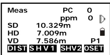
3. Press F4: [STOP] to finish measurement. The “SD”, “HD”, and “VD” will display as shown left.
