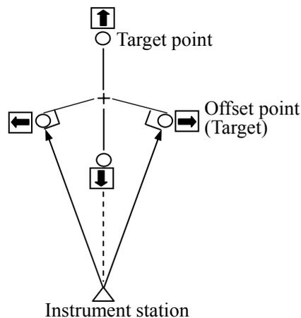
When the offset point is positioned to the left or right of the target point, make sure the angle formed by lines connecting the offset point to the target point and to the instrument station is almost  $90^\circ$ .
