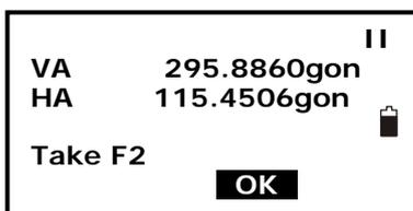
5. Sight the reference point in face II. Rotate the instrument  $180^\circ/200\text{gon}$  and sight the same point, then press F3: [OK].
