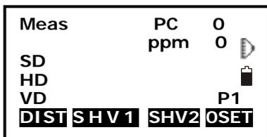
1. Aim at the target, press F3:[SHV2], the display mode of basic measurement will change to SD/HD/VD mode, and then press F1:[DIST] to start measure distance.
