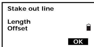
3. Input values of length and offset, then press F4: [OK], the coordinate of the required point is calculated and displayed.
