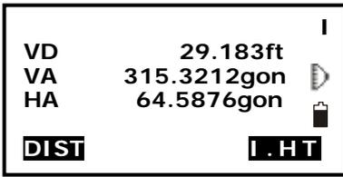
3. Aim at the target point and then press F1: [DIST]. You can press F4: [I.H.T] to re-input instrument height or target height here.
