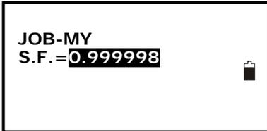
6. Input the scale factor if necessary. The range: 0.5000000 ~ 2.000000, and the factory setting is 1.000000.
