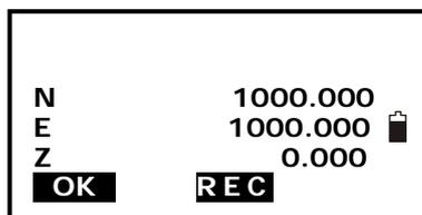
4. The calculated data displays. Press F3: [REC] to record it in the list, and press F1: [OK] back to menu mode.
