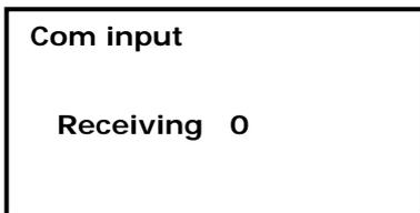
4. Run FOIF Exchange software PC, see the help file of FOIF Exchange to upload known data to current JOB, the chapter is “2.1.2 Upload Known data from PC to RTS100/RTS100R internal memory”.
