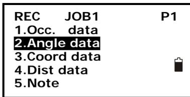
2. Select "2. Angle data", then aim at the target, the angle will display in real time.
