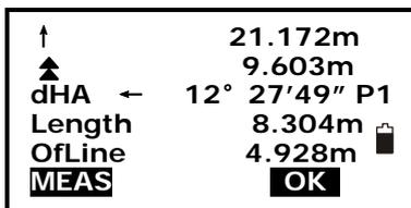
5. Press F1:[MEAS] to measure current rod, the staking data will display.
