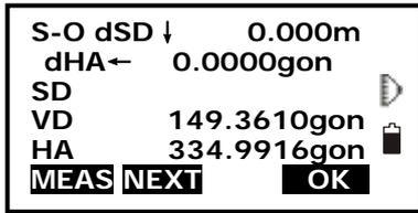
6. Horizontally rotate the instrument until “dHA” is near 0 and set the target on the sight line.
