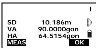
6. User could press F1: [MEAS] to re-measure the offset point or press F4: [OK] to the next step.
