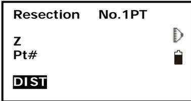
5. Sight the first known point and press F1: [DIST] to begin measurement. The measured data are displayed.
