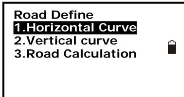
2. Select **1.Input the parameter** to enter road design menu. And then select **1.Horizontal Curve**, start point entering menu will display.
