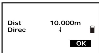
8. Press F4: [OK] to calculate and display the distance and angle of the target point.
