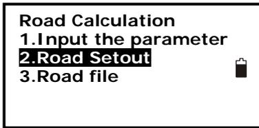
1. Press F2: [MENU] on P2 of the basic measurement mode, on the page 3 select **5.Road Calculation** enter road menu.
