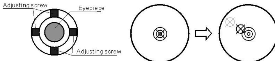
NOTE: When adjust the screws of plummet reticle, firstly loosen the screw on the moving direction of reticle, secondly tighten another screw by the same amount, clockwise turning is for tightening, and anticlockwise turning is for loosening, the turning amount for tightening or loosening should be same.
