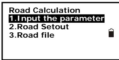
1. Press F2: [MENU] on P2 of the basic measurement mode, on the page 3 select **5.Road Calculation** enter road menu.
