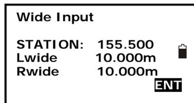
4. Input the parameters of road width.
