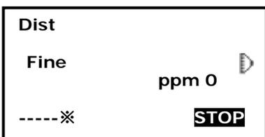
2. The symbol “\*” moves continually when measuring distance. Distance measuring mode, prism const and ppm value are also presented.
