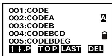
4. Press ▲ or ▼ key to move the cursor, and input or correct code.
