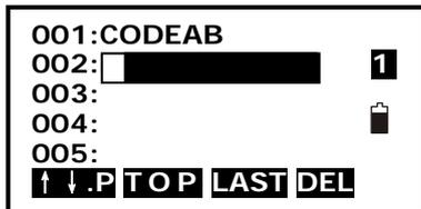
2. Input the code in turn and press the blue key {ENT} to save it. You can press key {BS} to delete your wrong input before the cursor. The max length of a code is 16 characters.
