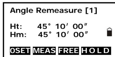
7. Recollimate the target A using the horizontal clamp and tangent screw, and press the F3:[FREE] key.
