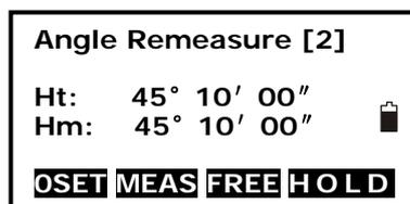
8. Recollimate the target B using the horizontal clamp and tangent screw, press the F4:[HOLD] key.
