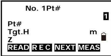
3. After setting the elevation for the first known point, press F3: [NEXT] to set the second point data.
