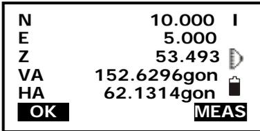
3. Press F4: [MEAS] to re-measure distance or press F1: [OK], the measured data is set as“Pt-01”.
