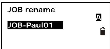
4. Input a new name and press key {ENT} to save the setting. The maximum length of a JOB name is 12 characters.
