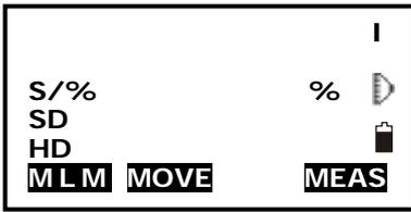
4. Aim at the next point P3 and press F1: [MLM] to begin measure. Repeat this operation to measure other target points.
