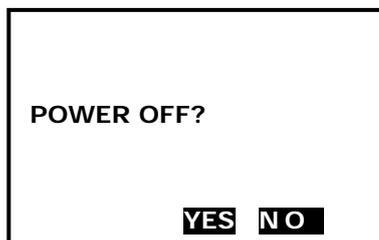
Press {POWER} key, the instrument will ask you to turn off the instrument or not, press F3(Yes), it will be turned off, press F4(No) back to previous screen.
