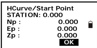
3. Enter the start point station and coordinate, press F4:[OK] key. Road horizontal elements editing menu will display.
