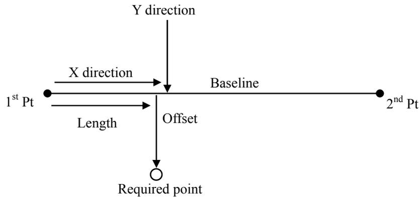
Length: Distance along the baseline from 1<sup>st</sup> point to the position at which a line extending from the required point intersects the baseline at right angles (X direction)
