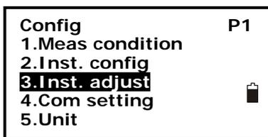
1. press F4: [CNFG] to enter into config mode.
