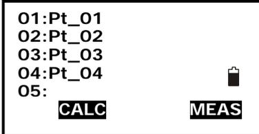
4. Repeat steps 2 and 3 till all points are measured one by one. Make sure measure them clockwise or anticlockwise. Press F2: [CALC] and the calculated area will display.
