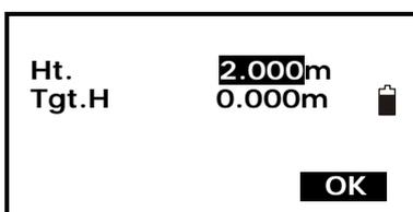
3. Input height from the surveying point to the position to be stake out. Then press F4: [OK] to set the data.
