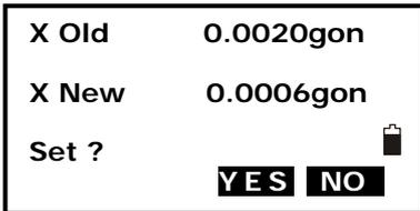
8. If both correction constant are in the range, press F3: [YES] to renew the correction angle, or press F4: [NO] to give up this adjustment,
