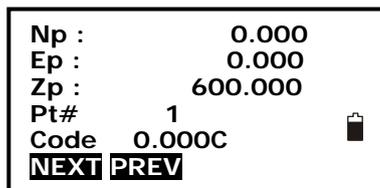
Code: Station mileage, “C” means center station, “R” means right station, “L” means left station.
