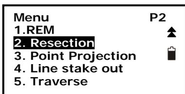
1. Press F2: [MENU] on P2 of the basic measurement mode, then press Func key to turn to page 2, and then select “7. Resection”, or press F4: [RES] at P3 directly.
