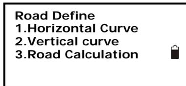
2. Press F4:[ENT] to calculate, “calculating” will display until “Cal complete” appear, the program go back to previous menu automatically.
