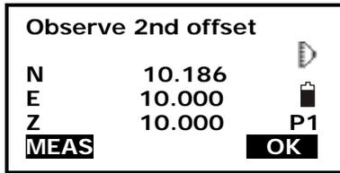
5. Sight the 2<sup>nd</sup> target, press F1: [MEAS] and measured data will display, press F4: [OK] to accept this value.
