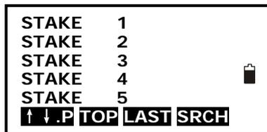
3. Select **3.Road data view** to view the staking station data, the station list will display.
