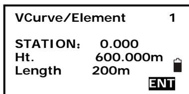
2. Press F4 to display Vertical road element inputting menu. Input the parameter for vertical element.
