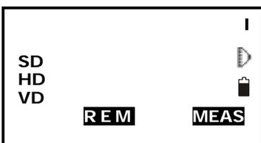
4. Aim at the target accurately and press F2: [REM]. The height from ground to the target is displayed in "Ht". Press F4: [MEAS] to repeat and press key {ESC} back to menu mode.
