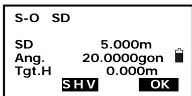
Press F2: [SHV] to shift between S-O SD, S-O HD, S-O VD.
