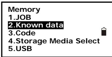
1. Connect instrument and PC via RS-232C communication cable. Press F3: [MEM] in the status mode to enter into memory management.
