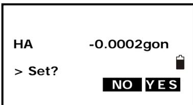
3. First aim the previous occupied point, then press F4: [YES] to set the previous foresight point coordinate as the occupied point coordinate or press F3: [NO] to give up.
