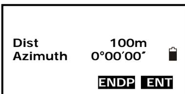
1. Make sure the instrument is in horizontal elements editing menu, press F2 to display line element inputting menu.
