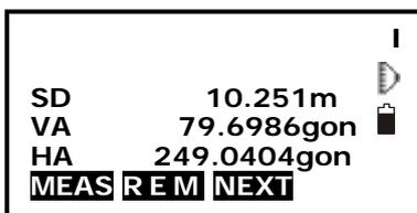
4. Press F2: [REM] to begin REM stake out measurement. Move telescope to find the point to be stake out.
