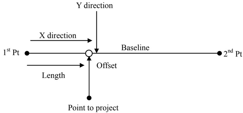
Length: Distance along the baseline from 1<sup>st</sup> point to 2<sup>nd</sup> point (X direction).
