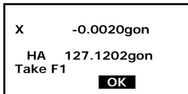
4. Wait a few seconds for this display to stabilize, then read the automatically compensated angles X1 and Y1.
