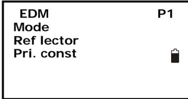
3. Change the settings if necessary. Press keys {▲}/ {▼} to select the first three items and press keys {◀} / {▶} to set the options.
