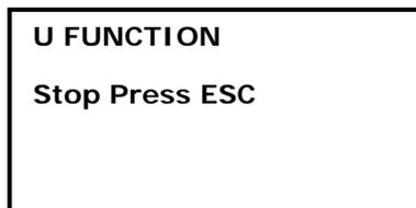
3. Connect instrument and PC via USB cable, RTS100/RTS100R series will display “U FUNCTION Stop Press ESC”. It means the RTS100/RTS100R is connected with PC already. Press [ESC] to disconnect them, and the instrument back to previous menu.
