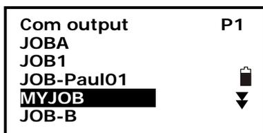
6. Press key {ENT} to start to send out via RS-232C port, it will back to JOB list mode after finishing.
