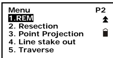
1. Set a target directly under or directly over the object and measure the target height with a tape measure etc.
