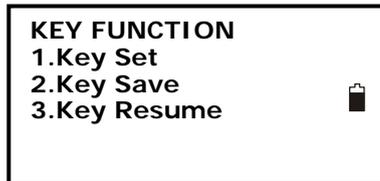
**Key Set: the soft key’s function at basic measurement mode can be changed**
