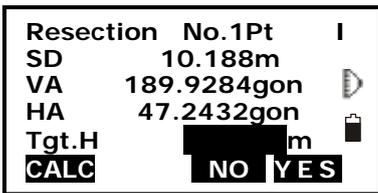
6. Press F1: [CALC] to calculate. Instrument occupied elevation and standard deviation are displayed.
