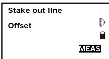
3. Input offset value: the horizontal move distance of baseline, right side indicates positive value and left side indicates negative value. Go to step 4 without inputting.
