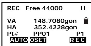
3. Press F4: [REC] to input the following items: point number, target height and code, press F1: [OK] to save data.
