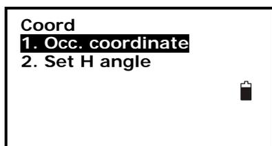
4. Select "1. Occ. coordinate" to input the occupied coordinates, instrument height and target height in corresponding field.
