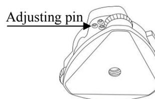
NOTE: Be careful when adjusting the three screws, and the tightening tension is identical for them.
