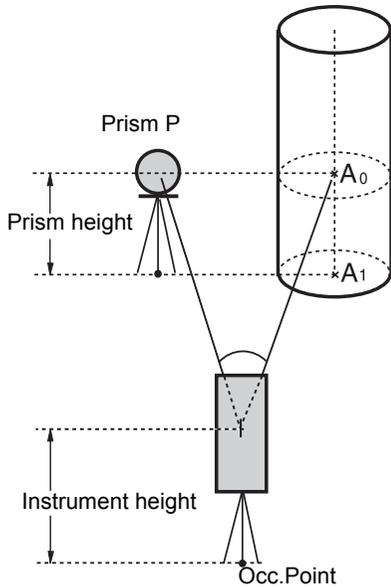
When measuring coordinates of ground point A1 :Set the instrument height / prism height.
