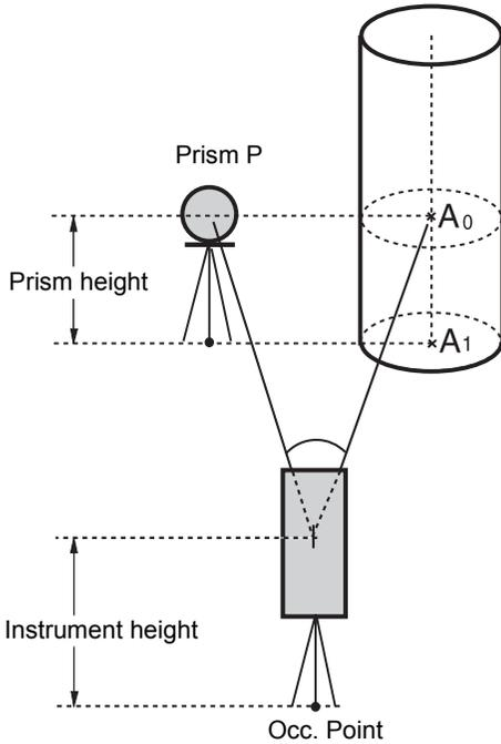
When measuring coordinates of ground point A<sub>1</sub> : Set the instrument height/prism height.
