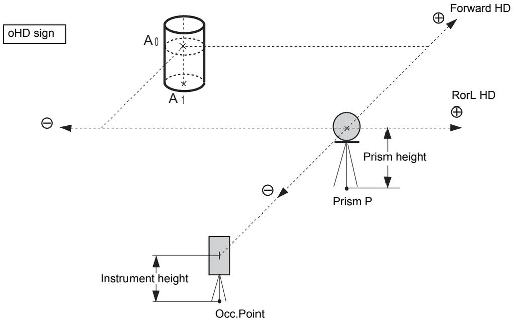
When measuring coordinates of ground point A<sub>1</sub>: Set the instrument height / prism height.
